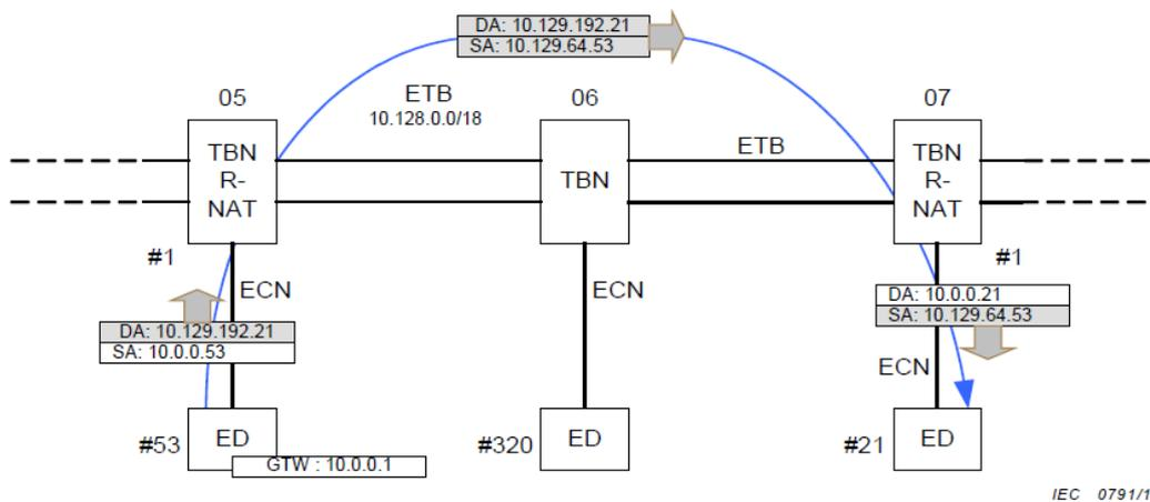
Figure 4 – An example of cross train-car communications
