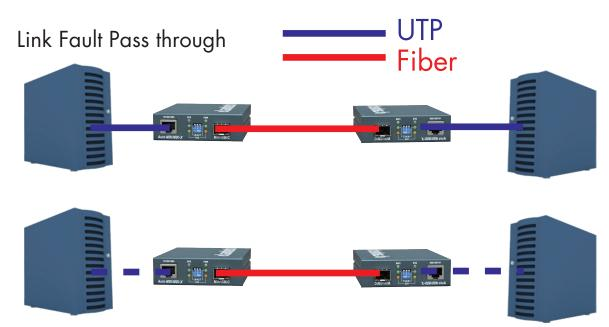
If Tx port link breaks down, it will force Tx port to disconnect.
