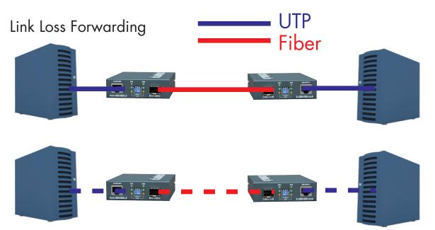
If Tx port link breaks down, it will force fiber port to disconnect.
