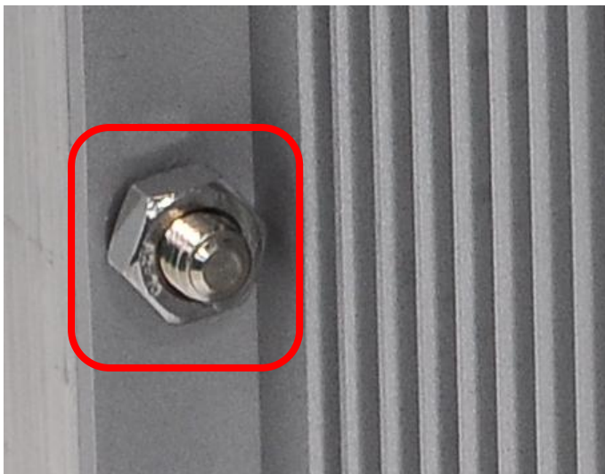
Ground screw of the switch
