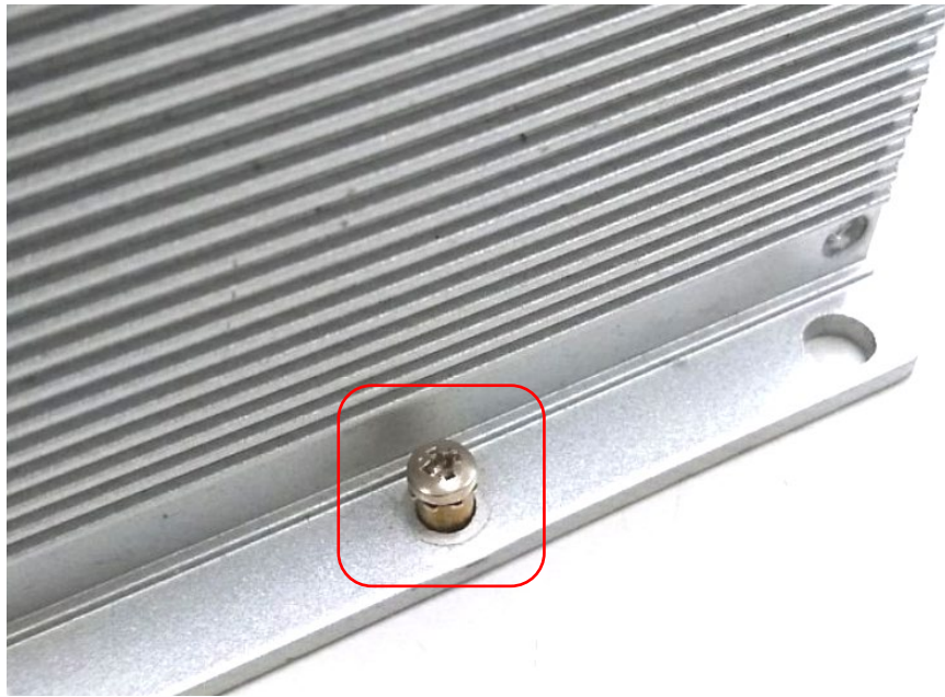
Ground screw of router
