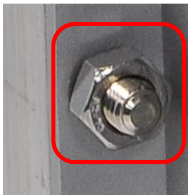
Ground screw of the switch
