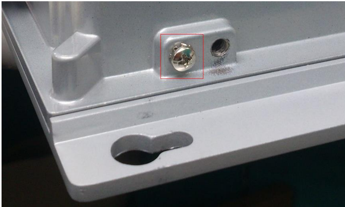
Ground screw of Ethernet switch
