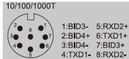
Pin assignment of M12 10/100/100T network connector (A-coded)
