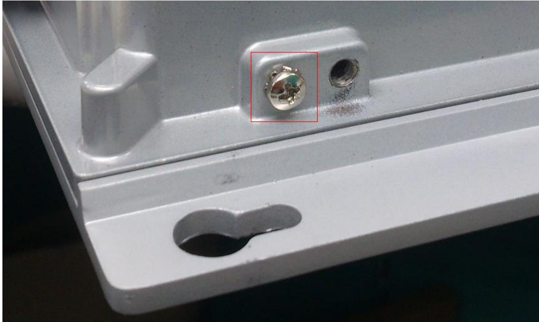
Ground screw of Ethernet switch
