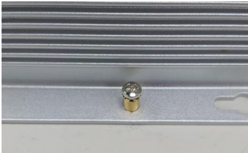
Ground screw of I(P)ES-5408T-IGN switch
