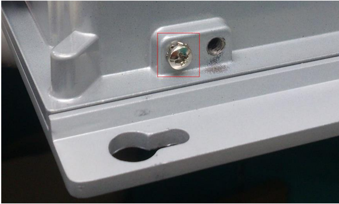
Ground screw of I(P)ES-0208 switch
