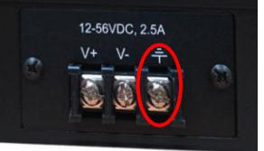
Make sure the grounding cable is attached between switch, power supply and earth.
