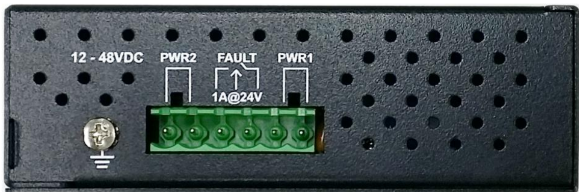
Bottom Panel of the industrial switch
