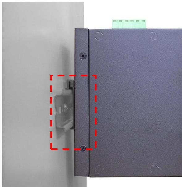
5. Check the DIN-Rail is tightly on the track.
