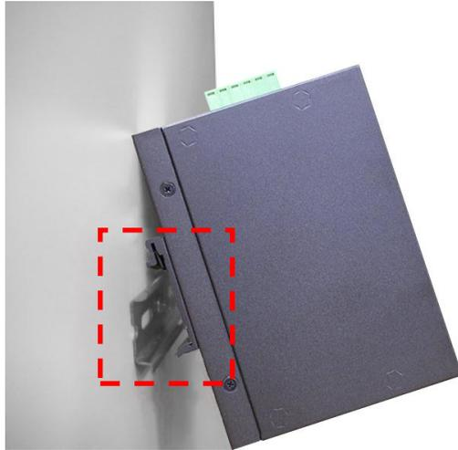
4. Then, lightly push the button of DIN-Rail into the track.
