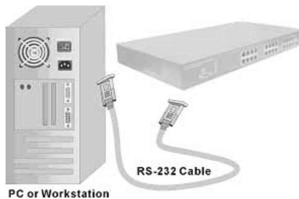
Connecting the switch to a terminal via RS-232 cable
